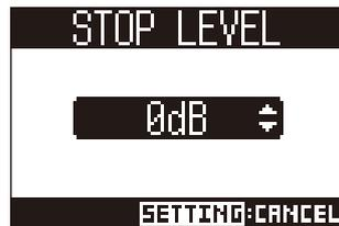
Recording will stop automatically when the level of the MASTER fader output stays below the set level for the amount of time set in step 4.
